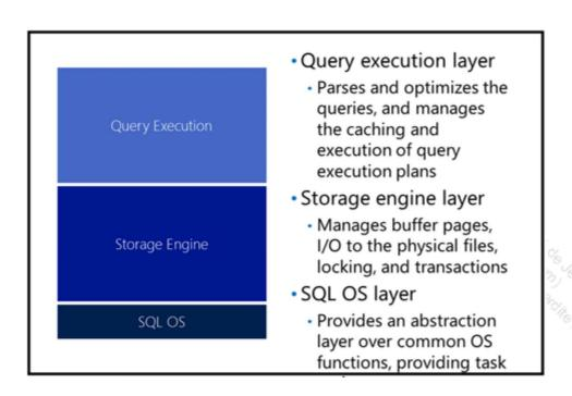
SQL Server is constructed from a series of many small components that work together. Three general categories of components exist within the database engine and are structured as layers – query execution (also referred to as the relational engine), storage engine, and SQL OS.
